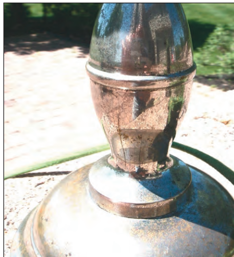
Due to a faulty annealing process, this Williams Abbott Potbelly has a few vertical cracks developing.
